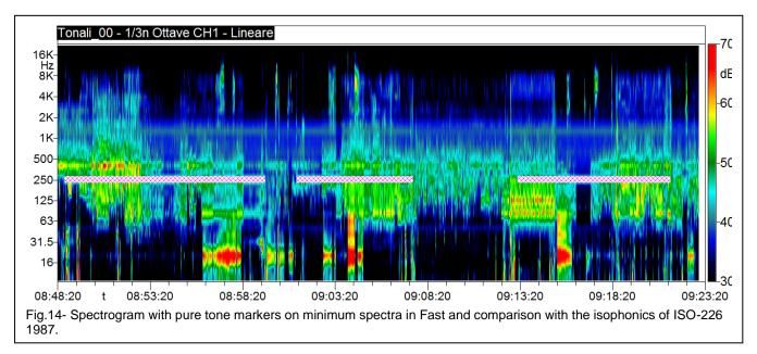
In the spectrogram of Fig.14, the research was instead conducted with the same settings as the previous analysis but now enabling the comparison with the isophonics of ISO-226 1987 as requested by the Ministerial Decree 16-03-98; the result now shows the presence of only the tonal component identified on the 1/3 octave band of 250 Hz, corresponding exactly to the noise of the recirculation pump being investigated and the markers precisely mark the periods of activity and pause.
