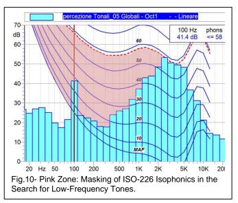
A similar situation can also be found when the tonal is at a higher frequency than those supported by the dominant equal-tone and it is sufficient for this tonal to be of an octave higher to have a distinct perception of it even for levels much lower than
