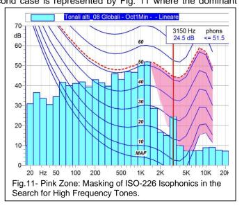
although this method has already been used in other applications, we have observed that in particular situations, it is of great help, especially when you have to examine long periods of time relating to measurements that come from unattended noise monitoring stations or in contexts where there may be tonal components coming from different sources that can manifest themselves with different durations and times.
