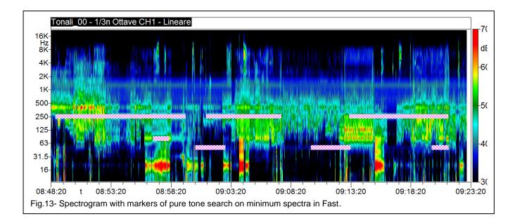
Looking at the tonal markers shown in Fig.13, it is noted that they identify multiple frequency bands, that the tonals are not continuously present, that in some periods more than one tonal may be present and that even in the presence of overlying environmental noise, the periods of presence of the tonals are identified with precision.
