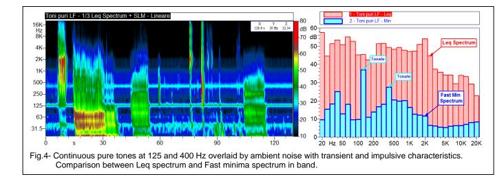
The situation described generates a Leq spectrum that does not allow the recognition of the presence of the tones that are present and clearly audible, while the spectrum of the minimums in the band is not influenced by transients or impulses and, being supported only by the components that are always present during the measurement, is able to show the presence of tones with continuous persistence.
