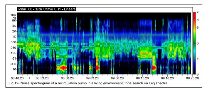
For this purpose, we have reported the example relating to the noise generated by a water recirculation pump of a condominium heating system, as it was detected inside an office, where employees said they were disturbed by this type of source. The situation is interesting because the pump does not work continuously and that in the office there are also various other possible sources of noise with tonal components that overlap with the noise generated by normal work activity.
