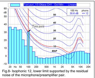
component were to drop in level, the residual noise of the microphone which can be seen gradually rising on the medium-high frequencies, would prevent its recognition.
