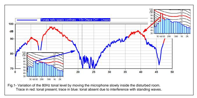
The example described in the graph in Fig.1 shows the time history of a tonal component located around 80 Hz in relation to a scan performed by moving the microphone slowly inside the disturbed environment; from the level profile over time, one can easily observe the variations introduced by the presence of standing waves, which exceed 20 dB and which indicate that in some points of the environment the tonal component at 80 Hz almost disappears.
