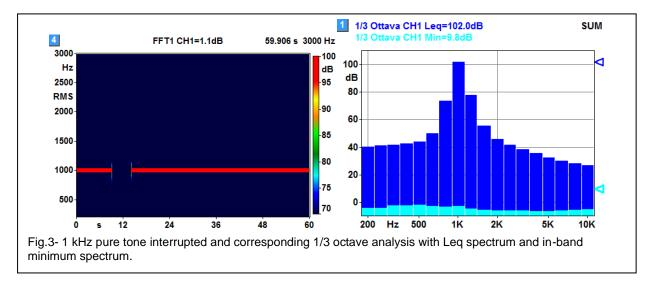
Differently, the spectrum of the minimums allows, compared to the corresponding Leq spectrum, the recognition of the presence of a tonal component even in the case in which other components should overwhelm or mask it for durations that can also be significant compared to the total measurement time.
